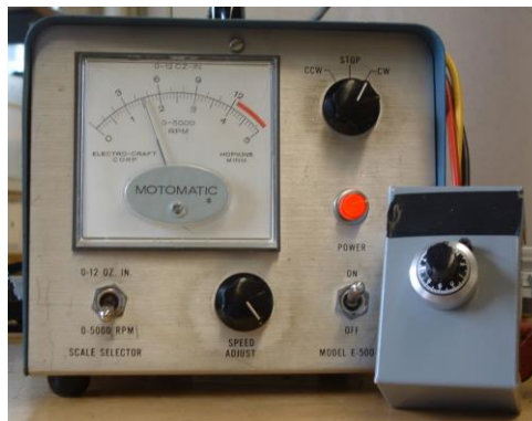
Figure 3. Motor Speed Control; use the knob on the small attached box, not on the motor.
