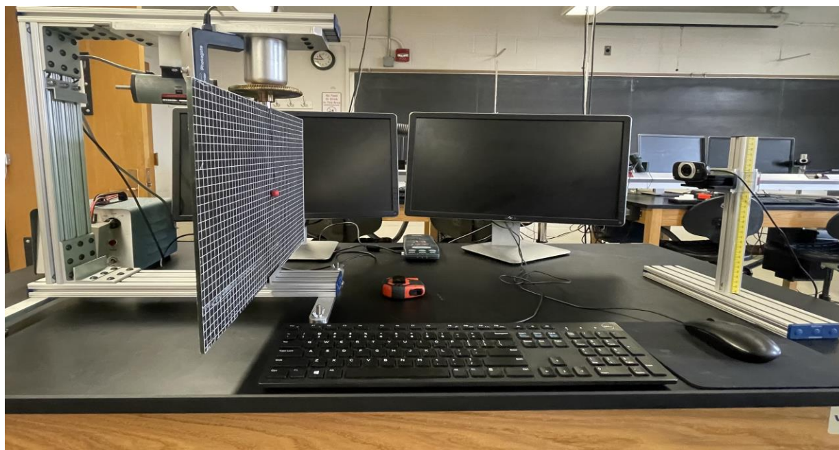
Figure 1. Photograph of the centripetal motion apparatus, motor controller and camera.
