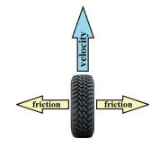
When are car turns, the tires can only exert a friction force on one side or the other. One side would have a friction component in the direction of motion (which is not allowed). The friction force is thus felt on the other side with two components. One component is perpendicular to the motion, causing the car to turn. The other is opposite the velocity, causing the car to decelerate.
