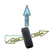
Note: Anti-lock brakes keep a car from skidding. Skidding cars are affected by the coefficient of kinetic friction, which is typically smaller than the coefficient of static friction. A non-skidding car affected by the larger static coefficient will stop faster.
