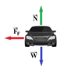
There are three forces acting on the car: the weight, the normal force, and the friction force.
