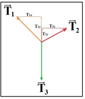
Start by making a force diagram for the hanging mass, labeling the tension in the line above it  $T_3$ . Then make a force diagram at the point of intersection of the three tensions.
