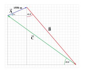
$A_{x} = (1550 \text{ m})\cos(25.0^{\circ}) = 1404.8 \text{ m}$   $A_{y} = (1550 \text{ m})\sin(25.0^{\circ}) = 655.1 \text{ m}$   $B_{x} = B \cdot \sin(41.0^{\circ}) \quad \{B_{x} \text{ is the opposite side}\}$   $B_{y} = -B \cdot \cos(41.0^{\circ}) \quad \{B_{y} \text{ is pointed down}\}$   $C_{x} = -C \cdot \cos(35.0^{\circ}) \quad \{C_{x} \text{ is pointed left}\}$   $C_{y} = C \cdot \sin(35.0^{\circ})$
