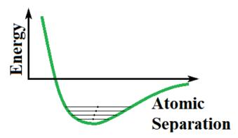
Each atom vibrates in a potential well created by its neighbors. Notice that the average separation (the center of the vibration) increases with energy due to the shape of the well.
