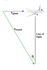
$$v_{airplane} = v_{sound} \sin \theta = \left(343 \frac{m}{s}\right) \sin 20.0^{\circ} = 117 \frac{m}{s}$$
