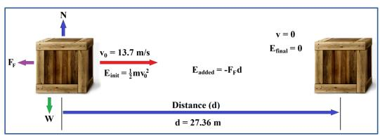
$$E_{init} = \frac{1}{2}mv_0^2 \qquad E_{final} = 0 \qquad E_{added} = -F_F d = -\mu_k N d = -\mu_k mgd$$
