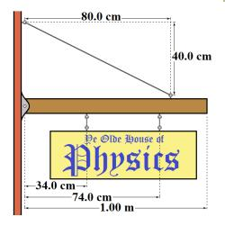
**Example**: A 2.50 kg sign is hung from an 11.0 kg beam as shown in the diagram. The sign is balanced so that half its weight is supported by each of the two wires above it. The beam is attached to the wall on the left by a frictionless pin that allows it to rotate and held in place by a guy wire above it. Determine the tension in the guy wire.
