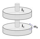
**Example**: A solid disk ( $I_1 = 4.00 \text{ kg} \cdot \text{m}^2$ ) is spinning about a fixed spindle at  $\omega_0 = 15.0 \text{ rad/s}$ . A second solid disk ( $I_2 = 6.00 \text{ kg} \cdot \text{m}^2$ ), which is not rotating, is placed on the spindle and dropped onto the first disk. There is friction between the two disks, and eventually they spin together. Determine (A) the velocity of the two discs once they start spinning together and (B) the energy is lost during the collision.
