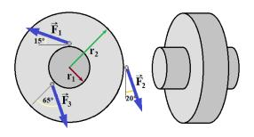
$$\sum \tau = \tau_1 + \tau_2 + \tau_3 = r_1 F_1 \sin 75^\circ - r_2 F_2 \sin 70^\circ + r_1 F_3 \sin 65^\circ$$
