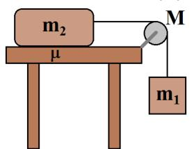
**Example**: A box of mass  $m_2 = 10.0$  kg sits on a table as shown. On one side a cord connects it to a hanging weight of mass  $m_1 = 25.0$  kg. The cord stretches over a frictionless pulley, a solid disk of uniform density with mass M = 5.00 kg. If the coefficient of kinetic friction between the box and table is 0.300, determine the acceleration of the box on the table.
