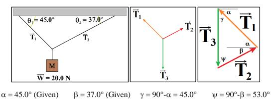
$$\frac{\sin \psi}{T_1} = \frac{\sin (\alpha + \beta)}{T_3} \qquad T_3 \cdot \sin \psi = T_1 \cdot \sin (\alpha + \beta)$$
