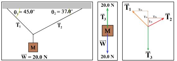
Start by making a force diagram for the hanging mass, labeling the tension in the line above it ' $T_3$ '. Then make a force diagram at the point of intersection of the three tensions. Break  $T_1$  and  $T_2$  into components. This is static equilibrium so the forces must equal  $\Sigma E_1 = 0$ .  $\Sigma E_2 = 0$
