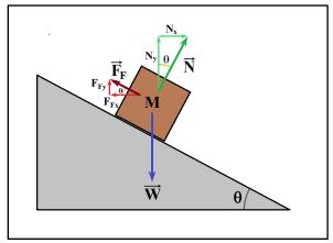
$N = Mg/[\mu_{S} \cdot Sin(\theta) + Cos (\theta)]$   $N = (10.0 \text{ kg})(9.80 \text{ m/s}^{2})[(0.57735) \cdot Sin(30.0^{\circ}) + Cos (30.0^{\circ})] = 84.8705 \text{ N} \implies 84.9 \text{ N}$   $F_{F} = \mu_{S} \cdot \text{N} = (0.57735)(84.8705 \text{ N}) = 49.0 \text{ N}$
