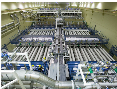
FIGURE 32.19 National Ignition Facility (CA). This image shows a laser bay where 192 laser beams will focus onto a small D-T target, producing fusion. (credit: Lawrence Livermore National Laboratory, Lawrence Livermore National Security, LLC, and the Department of Energy)
