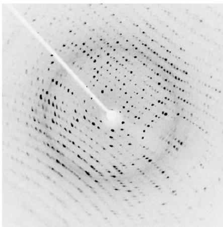
**FIGURE 30.27** X-ray diffraction from the crystal of a protein, hen egg lysozyme, produced this interference pattern. Analysis of the pattern yields information about the structure of the protein. (credit: Del45, Wikimedia Commons)
