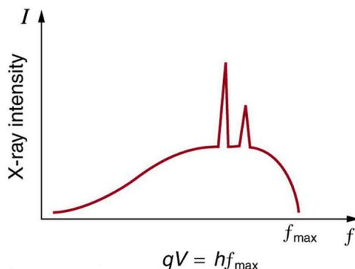
**FIGURE 30.20** X-ray spectrum obtained when energetic electrons strike a material, such as in the anode of a CRT. The smooth part of the spectrum is bremsstrahlung radiation, while the peaks are characteristic of the anode material. A different anode material would have characteristic x-ray peaks at different frequencies.
