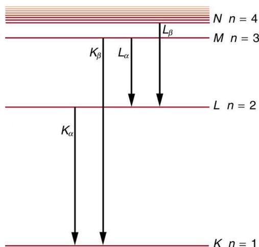
**FIGURE 30.21** A characteristic x ray is emitted when an electron fills an inner-shell vacancy, as shown for several transitions in this approximate energy level diagram for a multiple-electron atom. Characteristic x rays are labeled according to the shell that had the vacancy and the shell from which the electron came. A  $K_{\alpha}$  x ray, for example, is produced when an electron coming from the  $n = 2$  shell fills the  $n = 1$  shell vacancy.
