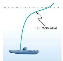
FIGURE 24.10 Very long wavelength radio waves are needed to reach this submarine, requiring extremely low frequency signals (ELF). Shorter wavelengths do not penetrate to any significant depth.
