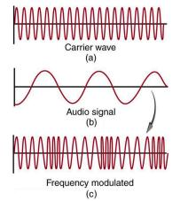
FIGURE 24.12 Frequency modulation for FM radio. (a) A carrier wave at the station's basic frequency. (b) An audio signal at much lower audible frequencies. (c) The frequency of the carrier is modulated by the audio signal without changing its amplitude.
