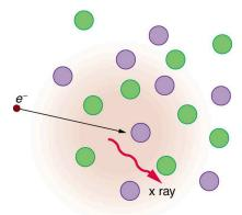
FIGURE 24.19 Artist's conception of an electron being slowed by collisions in a material and emitting X-ray radiation. This energetic electron makes numerous collisions with electrons and atoms in a material it penetrates. An accelerated charge radiates EM waves, a second method by which X-rays are created.
