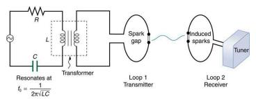
FIGURE 24.4 The apparatus used by Hertz in 1887 to generate and detect electromagnetic waves. An *RLC* circuit connected to the first loop caused sparks across a gap in the wire loop and generated electromagnetic waves. Sparks across a gap in the second loop located across the laboratory gave evidence that the waves had been received.
