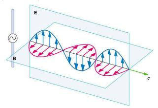
FIGURE 24.7 A part of the electromagnetic wave sent out from the antenna at one instant in time. The electric and magnetic fields (E and B) are in phase, and they are perpendicular to one another and the direction of propagation. For clarity, the waves are shown only along one direction, but they propagate out in other directions too.
