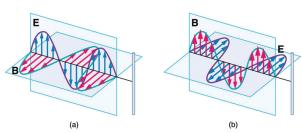
FIGURE 24.23 Electromagnetic waves approaching long straight wires.
