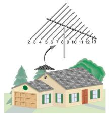
**FIGURE 24.26** A television reception antenna has cross wires of various lengths to most efficiently receive different wavelengths.
