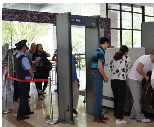
FIGURE 23.41 The familiar security gate at an airport can not only detect metals but also indicate their approximate height above the floor. (credit: shankar s/Flickr)
