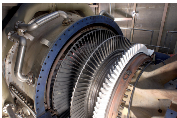
FIGURE 23.23 Steam turbine/generator. The steam produced by burning coal impacts the turbine blades, turning the shaft which is connected to the generator. (credit: Nabonaco, Wikimedia Commons)
