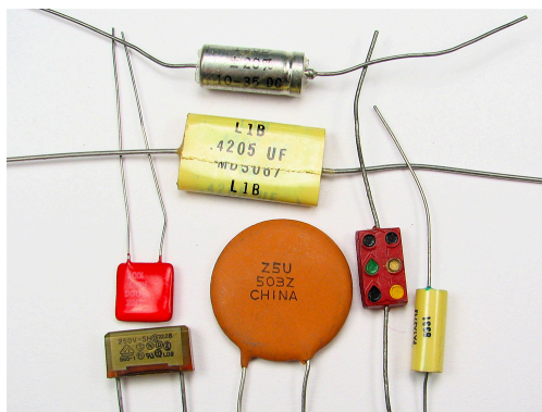
FIGURE 19.14 Some typical capacitors. Size and value of capacitance are not necessarily related. (credit: Windell Oskay)
