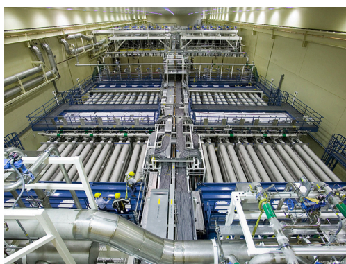
Figure 32.21 National Ignition Facility (CA). This image shows a laser bay where 192 laser beams will focus onto a small D-T target, producing fusion. (credit: Lawrence Livermore National Laboratory, Lawrence Livermore National Security, LLC, and the Department of Energy)
