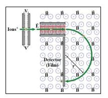
① Ions from source (sample) are accelerated through a potential V.
