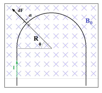
Straight Sections:  $F = ILBSinq = ILB_0$ These point in opposite directions (cancel) Curved Sections:  $dF = IBSinqdL = IB_0dL$   $dF = vector \rightarrow Must sum components$ x-components will cancel (symmetry)  $\left|\vec{F}\right| = F_y = \int_0^{\pi} dF \cdot Sin\phi = \int_0^{\pi} IB_0 \cdot Sin\phi \cdot dL$   $\left|\vec{F}\right| = \int_0^{\pi} IB_0 Sin\phi \cdot Rd\phi = IB_0 R \int_0^{\pi} Sin\phi d\phi$  $\left|\vec{F}\right| = IB_0 R [-Cos\phi]_0^{\pi} = 2IB_0 R$
