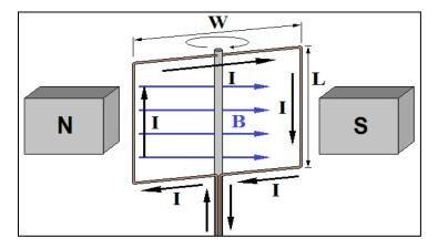
If we send current through the loop the magnetic field creates torque, turning the loop. This is a **motor**.
