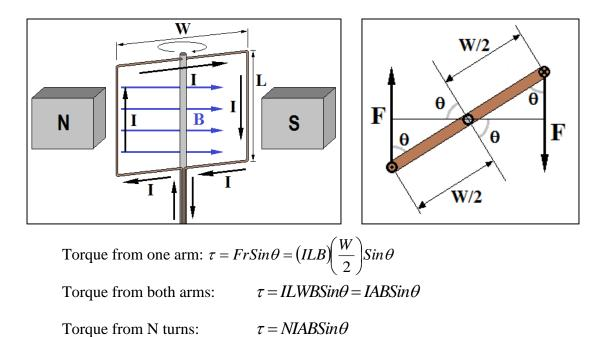
Magnetic Dipole Moment:  $\vec{\mu} = NI\vec{A}$   $\vec{\tau} = \vec{\mu} \times \vec{B}$
