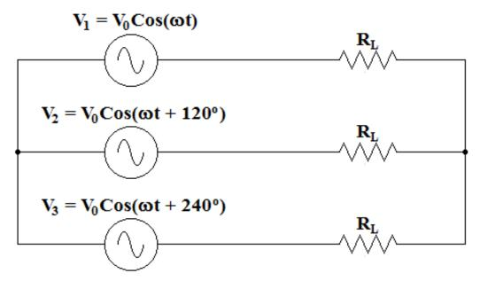
By symmetry the connecting point on the right must be a ground (no ground wire needed!)
