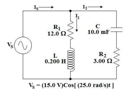
$Z_{EO} = 4.324\Omega\angle - 34.32^{\circ} = 3.751\Omega - i2.438\Omega$
