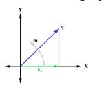
If you take a vector of magnitude V and let it rotate at constant angular frequency ( $\omega$ ), the x-component of the vector will be: V<sub>X</sub>=V·Cos ( $\theta$ ) =V·Cos ( $\omega$ t+ $\theta_0$ )
